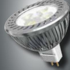
With a lighting power of more than 100Lm/Watts, the LED Spot complies with usual halogen lamps of the type MR16 in the power range of 35-50W. By comparison with halogen lamps, the extremely low heating of the housing permits the mounting also even where halogen lamps are not allowed to be used due to the heat development.
